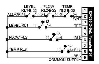
Dependent on your product type, signals will either be accessible via a standard two-row 9-pin D subminiature connector (see below left) OR direct connection to terminal blocks (see below right). Where a D connector is provided, the female gender (ATC PN EA096) is supplied in all cases. If male pins are required, we recommend using a male-to-male gender-changer connector (ATC PN EA853). Pin numbers are clearly marked on the molding. The connector is rated to IP67.
