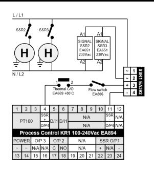
In the above, the low voltage control SSR has a contact side capable of supporting the current pulled by two heaters in parallel.
