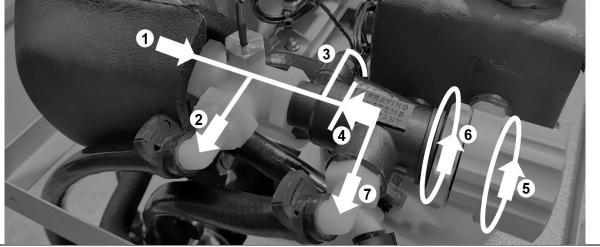
It is important to understand the basic principle that all else being equal, higher flow results in a higher demand for pressure. The motor generates the power required to turn the pump head and create that pressure. The more restrictive a water circuit is, the higher the pressure required to maintain flowrate. Positive displacement pumps are designed to generate high pressure and are mechanically tight - their RPM dictates flowrate. See image above.
